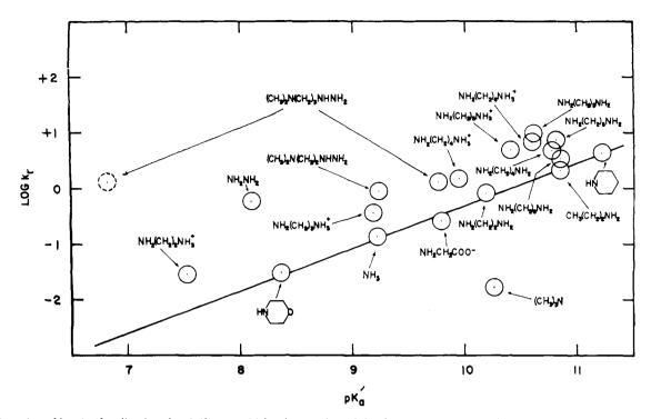
Figure 2. Plot of log  $k_r$  (for diamines log  $k_r/2$ ) vs.  $pK_a'$  for the reaction of simple primary and secondary amines,  $\alpha, \omega$ -diaminoalkanes, and  $\alpha, \omega$ -dimethylaminoalkylhydrazines with phenyl acetate (25°, H<sub>2</sub>O,  $\mu = 1.0 M$  with KCl).
